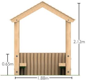
Large Toddler Shelter Seats constructed using 195 x 95mm sleepers. Shower proof roof constructed using shiplap boards. Size: 1.94m x 1.88m x 2.12m.
